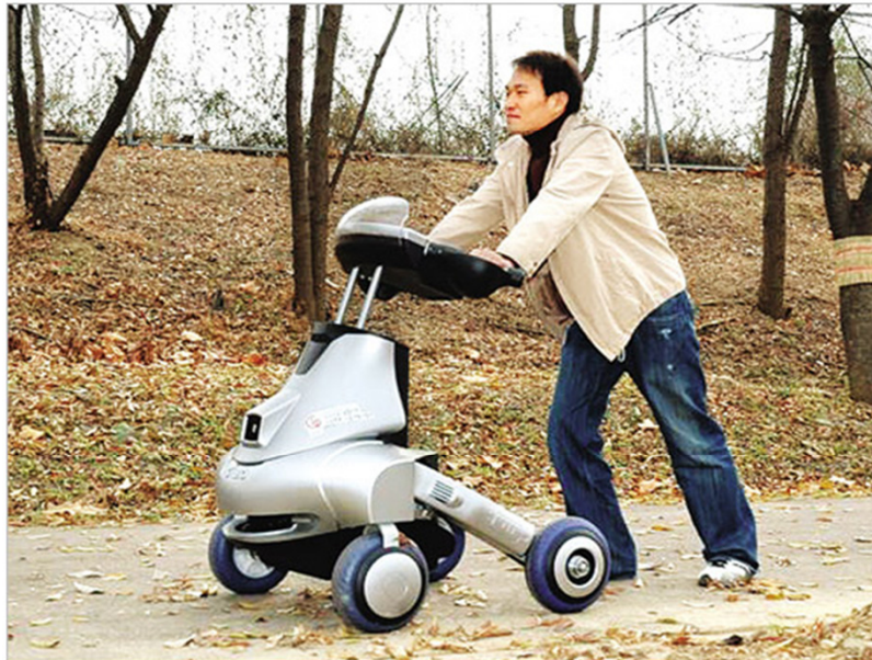
Korean Center for Intelligent Robotics outdoor assistive walking system
